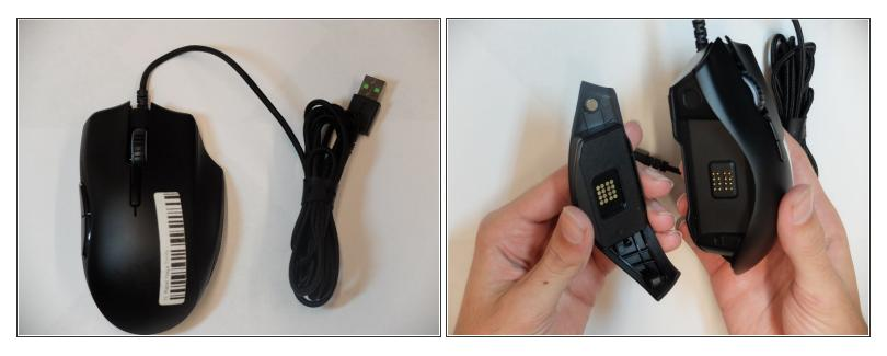
• Remove the interchangeable side plate.
