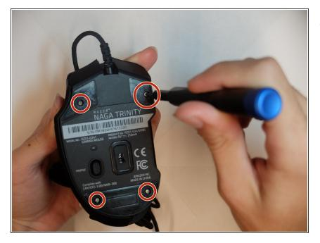
• Remove the four 6mm screws by using a JIS #1 screwdriver.
