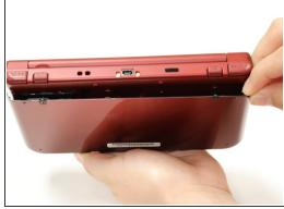
Wedge the opening pick in the cutout to separate the back plate from the device.
