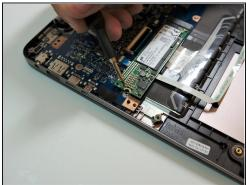
Unscrew the single 3.7mm screw holding down the M.2 SSD using the Philips #0 screwdriver bit.
