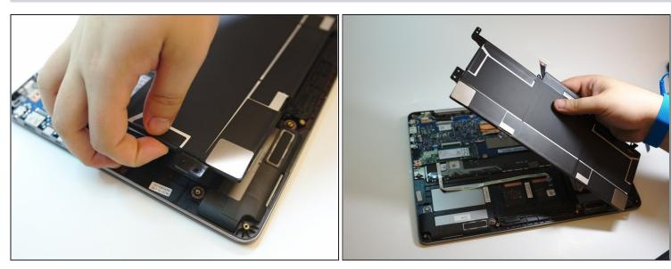
• Gently lift the battery out of the chassis of the device.
