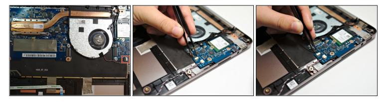
• Use the blunt nose tweezers to pull out the fan connector from the connector slot labeled 'FAN' on the right-hand mother board.
