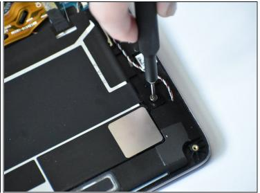
• Unscrew the six 3.7mm screws using the Philips #0 screwdriver bit.
