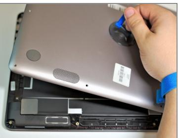
• Press the suction handle on the center of the back cover, and gently lift up.
