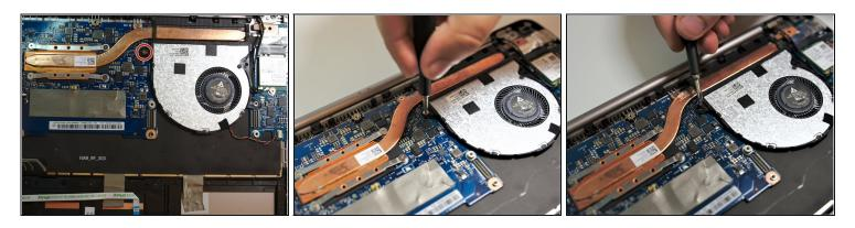
• Use the Philips #0 screwdriver bit to remove the 2.7 mm screw holding the fan.
