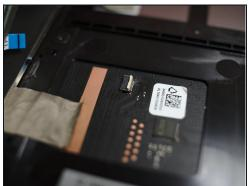
• Using the tweezers again, pull on the blue plastic tab with "TP" printed on it.
