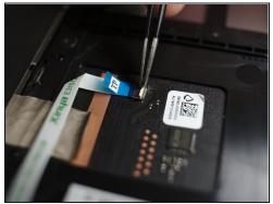
Use the tweezers to unlatch the clasp holding the ribbon cable
