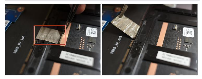
• Remove the strip of tape by grabbing the end of it with the blunt nose tweezers and pulling back.
