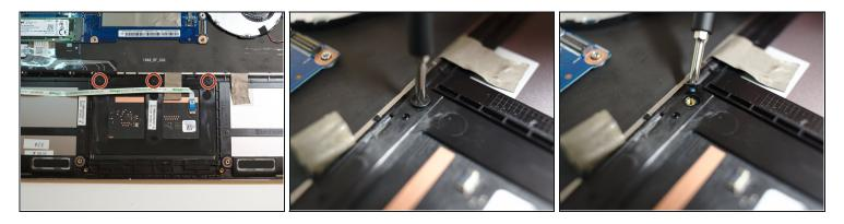
• Remove the three 2.5 mm screws across the top of the trackpad with the Philips #0 screwdriver.
