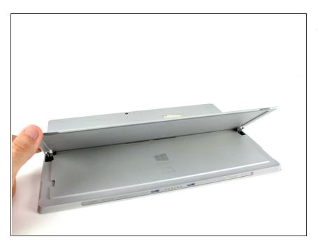
• Lift the kickstand to a 90° angle to expose the hinge screws.
