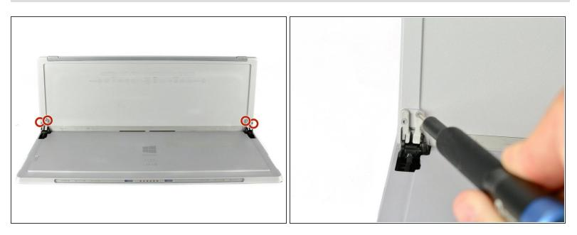
Remove the four 3.5 mm T5 screws—two on each side.
