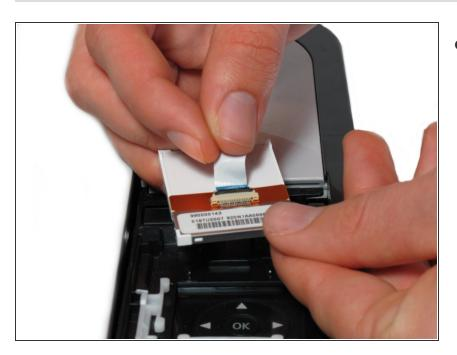
Completely remove the LCD by disconnecting the ribbon cable with a gentle pull.
