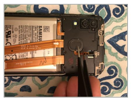
• Disconnect the Fingerprint scanner.
