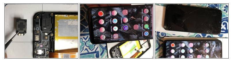
• Once you have completed the component removal, you can begin the reassembly by placing the components on the new display.
