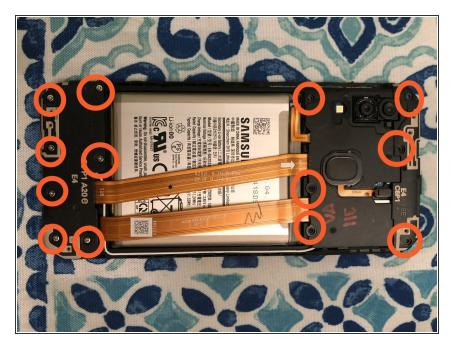
Using a Philips #00 screwdriver, remove the 13 screws securing the inner cover.
