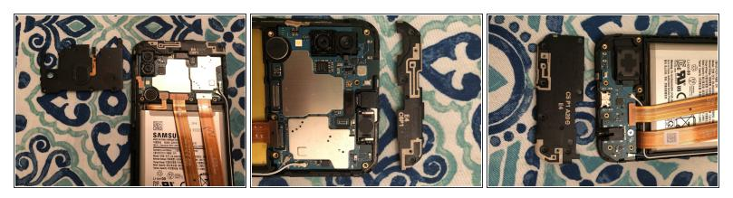
Now you can remove the upper and lower covers that protect the logic board and the speaker respectively.
