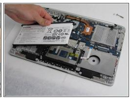
• Use a spudger to pry the battery connecting cable from the laptop and remove the battery.
