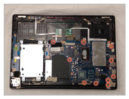
Using the Phillips #00 screwdriver, remove the ten 4mm screws.
