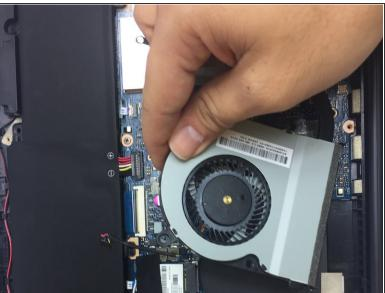
Once all screws and the connector are removed, you can safely pull the fan out of its place.
