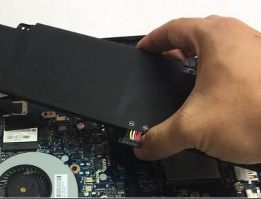
Once the screws and connector are removed, simply pull out the battery from its place.
