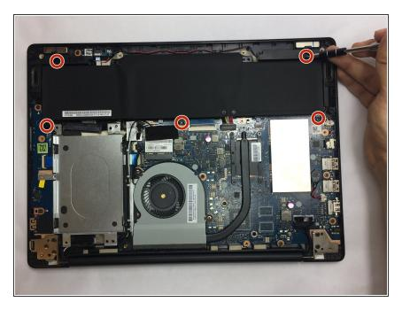
Use a Phillips #0 screwdriver and remove all five 5 mm screws securing the battery.
