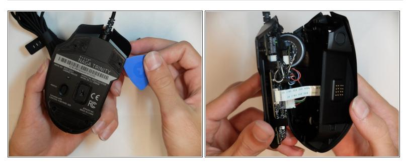
• Separate the top mouse housing from the bottom mouse housing using the opening pick.
