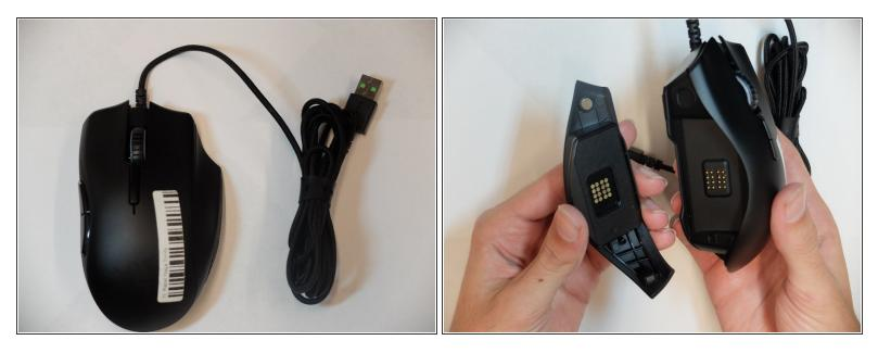
• Remove the interchangeable side plate.
