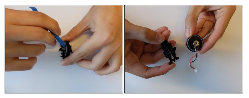
• Remove the scroll wheel from the scroll wheel housing using the opening tool.
