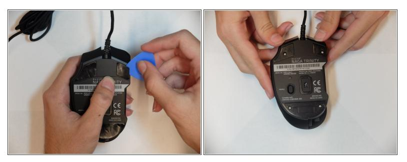
• Remove the mouse's feet using the opening pick.
