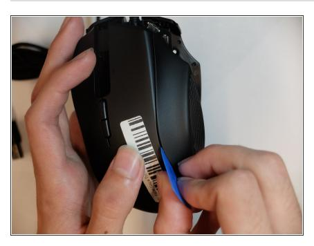
• Remove the side housing using the opening pick.
