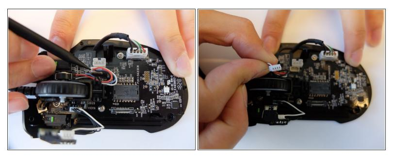
Remove the scroll wheel optical encoder 3-pin connector from the main board by wiggling the connector upwards.
