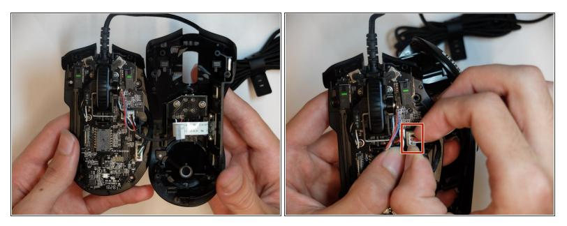
• Remove the top housing LED 3-Pin connector that is near the main board.
