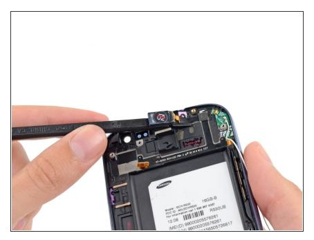
Use the flat edge of a spudger to peel the top portion of the earpiece/volume buttons/ambient light sensor ribbon cable from the front panel assembly.
