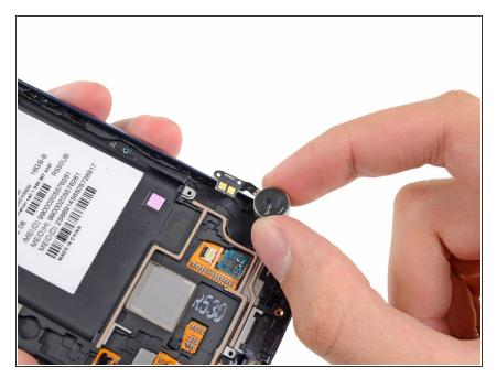
Lift and remove the vibrator out of the front panel assembly.
