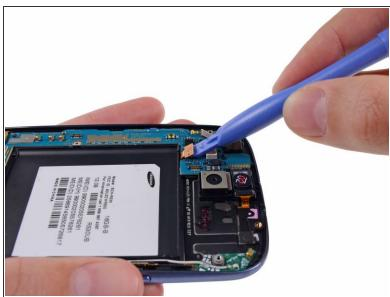
• Disconnect the digitizer cable by gently prying its connector up from its socket on the motherboard.
