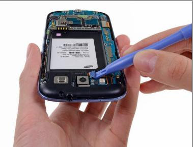
Use a plastic opening tool to pry the rear-facing camera connector up from its socket on the motherboard.
