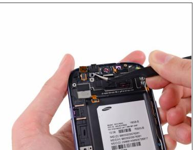
• Use a pair of tweezers to lift the front-facing camera/ambient light sensor/rear microphone assembly out from its socket in the front panel assembly.
