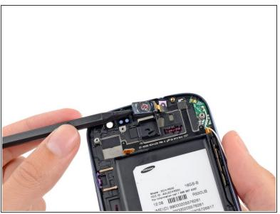
Wedge the tip of a spudger underneath the earpiece speaker and pry the earpiece speaker out of its recess in the front panel assembly.
