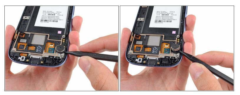
Use the tip of a spudger to pry the vibrator out of its recess in the front panel assembly.
