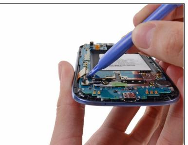
Disconnect the display data cable from the motherboard.
