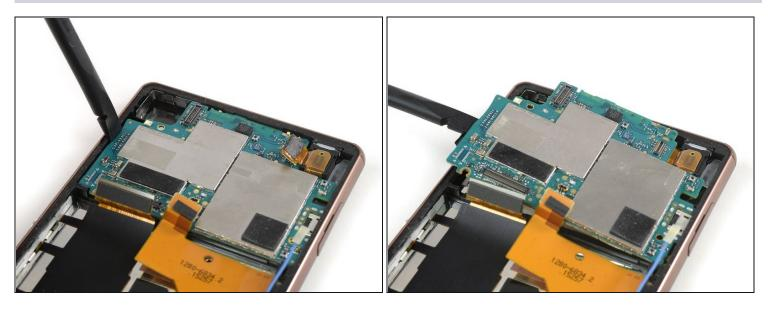
• Insert the flat end of a spudger into the gap between the midframe and the left edge of the motherboard.
