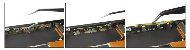
• Use a pair of tweezers and carefully pry the top left part of the main flex cable away from the midframe.
