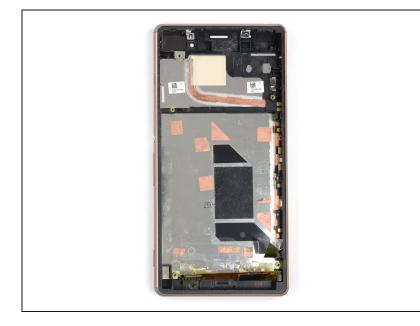
Compare your new replacement part to the original—you may need to transfer remaining components such as the protective foil in the earpiece speaker recess or remove adhesive backings from the new part before installing.
