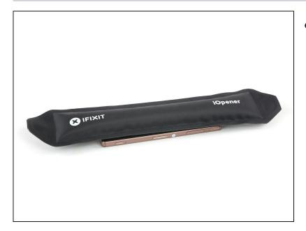
• Flip the phone over and apply a <u>heated iOpener</u> to the right side of the screen to loosen the adhesive beneath the main flex cable. Apply the iOpener for at least two minutes.
