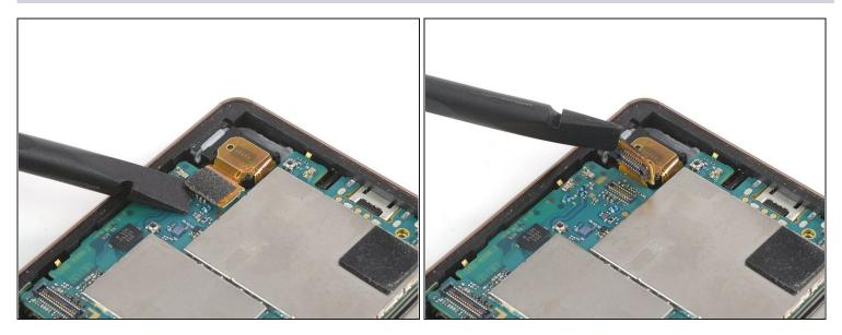
• Use a spudger to pry up and disconnect the headphone jack and microphone flex cable in the top right corner.
