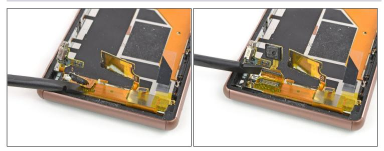
• Use a spudger to pry up and disconnect the main flex cable from the display flex connector located at the bottom of the phone.
