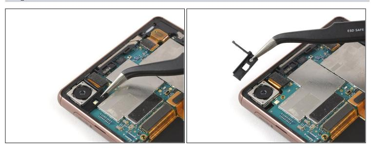
• Use a pair of tweezers to remove the black plastic bracket below the camera in the top left corner of the phone.
