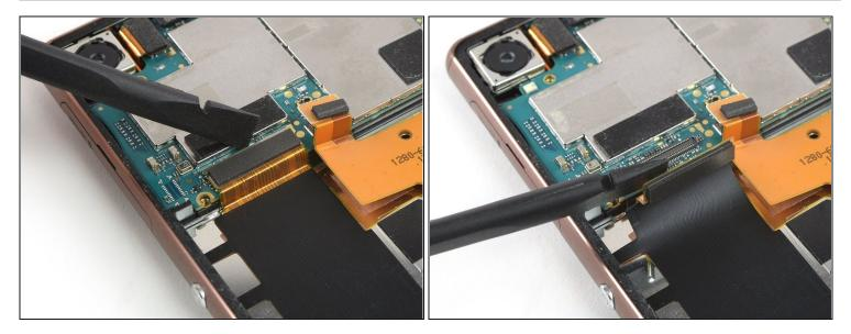
• Use a spudger to pry up and disconnect the main flex cable.
