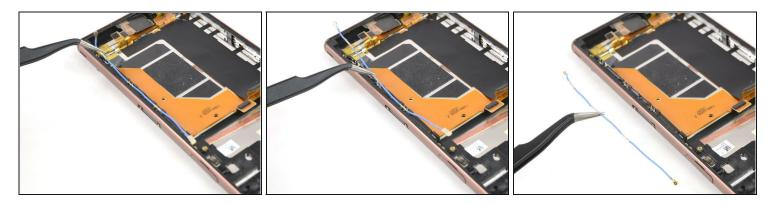
• Use a pair of tweezers to pry the blue antenna cable out of the brackets on the edge of the phone and remove it.
