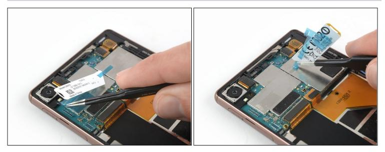
• Use a pair of tweezers to peel the blue foil off the motherboard.
