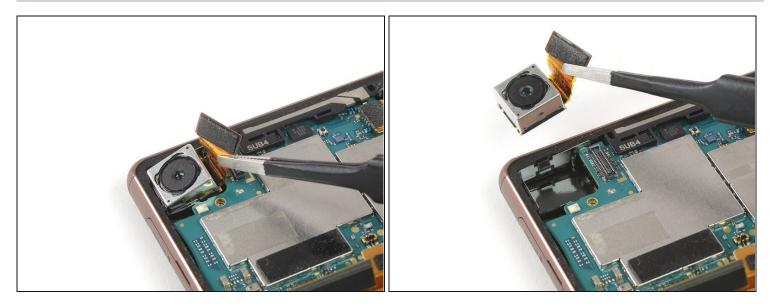
• Use a pair of tweezers to lift the rear camera out of its recess and remove it.
