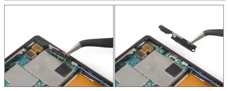
• Use a pair of tweezers to remove the black plastic cover from the right edge of the motherboard.
