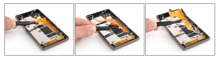
• Carefully peel the magnetic charging cable off the midframe and remove it.
