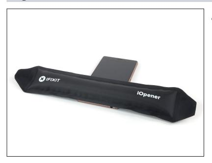
• Apply a <u>heated iOpener</u> to the upper end of the screen to loosen the adhesive beneath the headphone jack. Apply the iOpener for at least two minutes.
