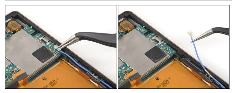
• Use a pair of tweezers to carefully pry up and disconnect the antenna cable at the bottom right of the motherboard.
