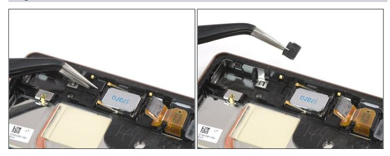
• Use a pair of tweezers to remove the black plastic spacer next to the earpiece speaker.
