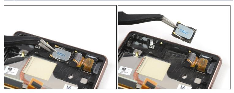
• Use a pair of tweezers to remove the earpiece speaker by carefully prying it out from its left where the spacer was before.
