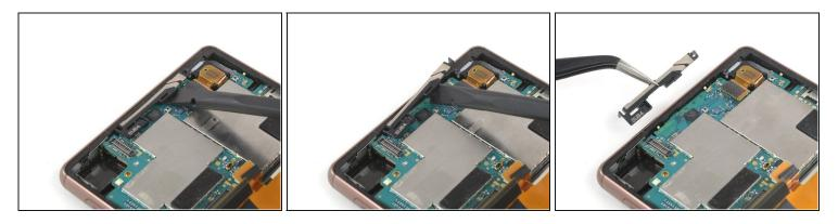
• Use a spudger to pry up the plastic cover at the top edge of the motherboard and remove it with a pair of tweezers.
