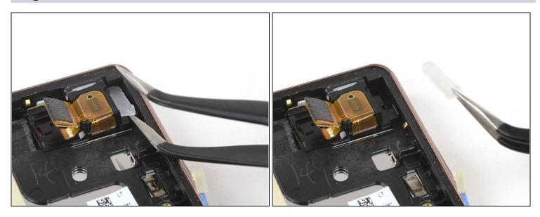
• Use a pair of tweezers to pry up and remove the white plastic piece next to the headphone jack.
