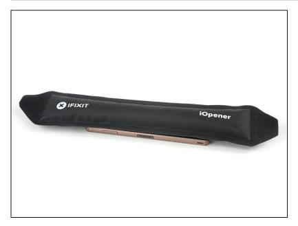
• Apply a <u>heated iOpener</u> to the left side of the screen to loosen the adhesive beneath the magnetic charging cable. Apply the iOpener for at least two minutes.
