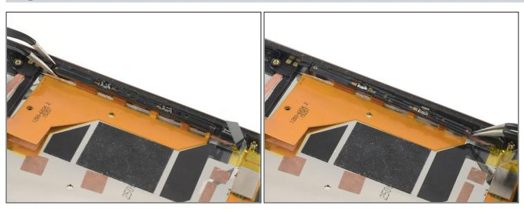
• On the right edge of the phone use a pair of tweezers to pry the magnetic charging cable out of its recess.
