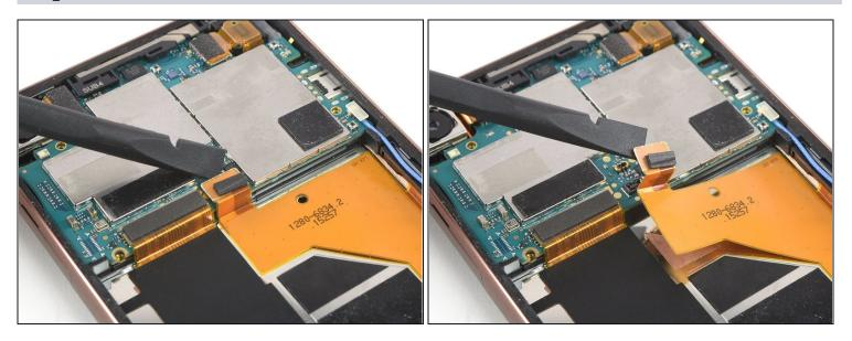
• Use a spudger to pry up and disconnect the magnetic charging flex cable
