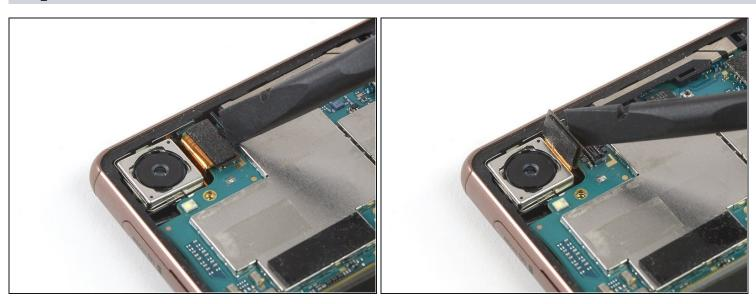
• Use a spudger to pry up and disconnect the rear camera flex cable.
