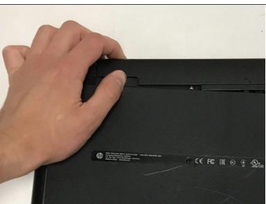
To remove the battery, slide the left slider on the back to the unlocked position.
