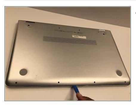
Go slowly around the edge with the opening tool. The noises you will hear are due to the small joints popping open. Continue this until you have made your way around the entire laptop.
