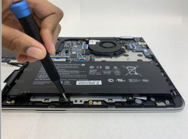
Remove the six 4mm screws around the battery using a Phillips #0 screwdriver.
