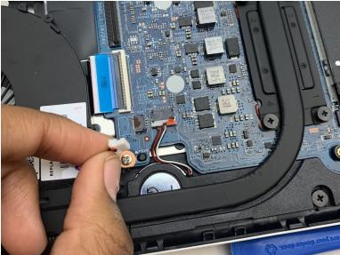
Disconnect the port with the red, yellow, and black wires by removing the wires with your fingers.
