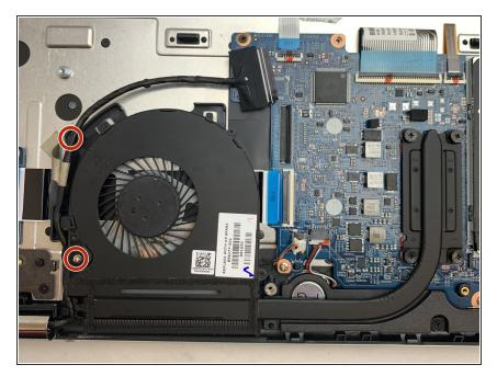
Remove the two 4.5mm Phillips #1 screws.
