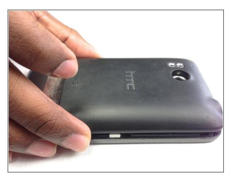
Lift and remove the rear panel.
