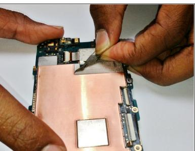
Use a finger nail to get in between the tape and the phone, then pull the tape off gently.
