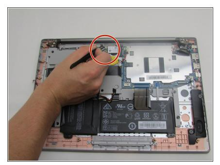
Remove the wireless card by disconnecting the two antenna cables and removing the 2.5 mm Phillips #0 screw.
