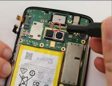
• Remove the two black 2.7 mm screws from the motherboard.
