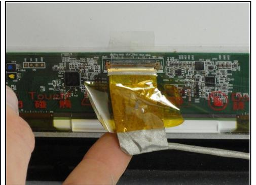
**⚠ Do not pull too hard to avoid damage to the connections.**
