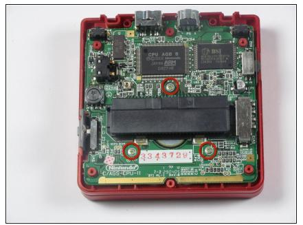
Using a Phillips #00 screwdriver, remove the three Phillips #00 4 mm long screws that hold the motherboard to the button panel.
