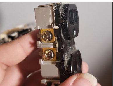
Hold the outlet with face of the outlet pointing toward you, with the copper screws on the right, and the silver screws on the left.
