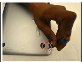
Remove the two 6mm JIS #0 screws from either side of the hinges.
