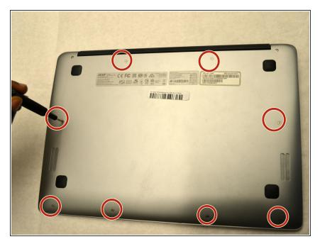
Remove the eight 4mm JIS #0 screws from the back cover.
