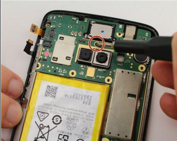
Remove the two black 2.7 mm screws from the motherboard.
