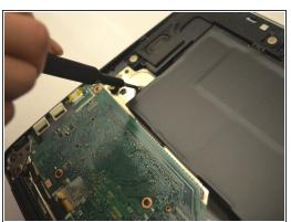
Remove the two JIS #0 screws that connect the battery to the rest of the laptop.
