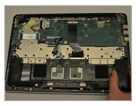
Lift the speakers from the frame, making sure to carefully unwind the wires connecting the speakers.
