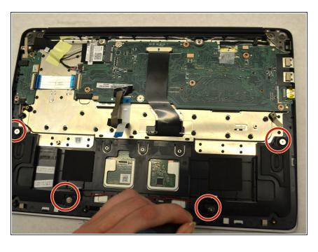
Remove the four 4mm JIS #0 screws that hold the speakers in place.
