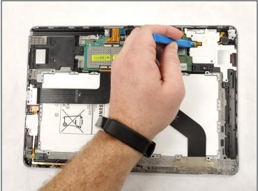
• Disconnect the five base connectors from the motherboard by using the blue opening tool to carefully remove the connectors.
