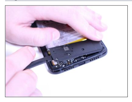
Use a spudger to lift and remove the speaker.
