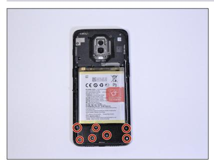
Remove seven 3mm Phillips #00 screws from the speaker.
