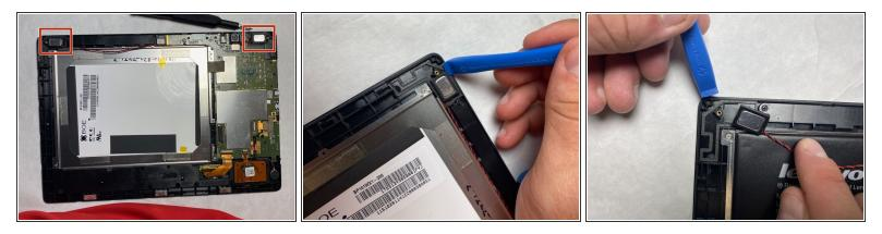
Use an opening tool to pry the speakers out of the tablet.
