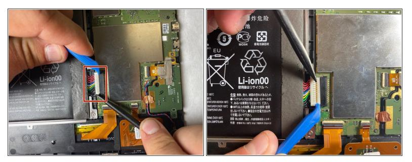
Using either the plastic opening tool or your fingers, gently pull on both sides of the plug to release it.
