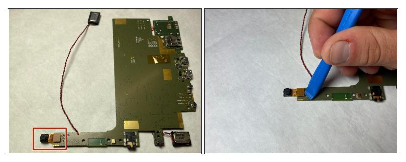
• Gently remove the front camera by pulling the ribbon connector out with a plastic opening tool.
