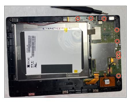
Remove the 3.2mm screws using a Phillips #000 screwdriver.
