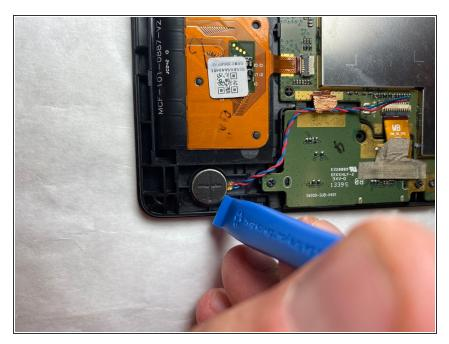
• Use the plastic opening tool to gently pry up the vibration motor.
