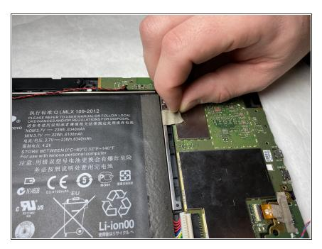
• Remove the piece of tape by pulling up with your fingers.
