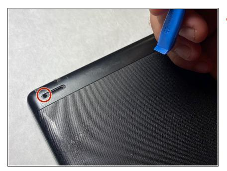
Remove the screws from both of the spots that were covered with a Phillips #000 screwdriver.
