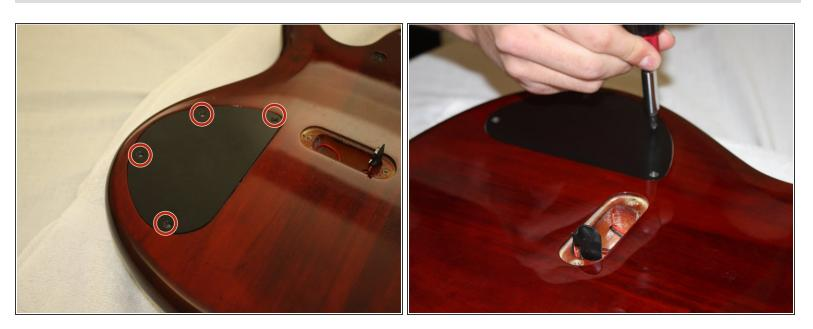
Use a Phillips #2 screwdriver to remove the four screws on the backplate.
