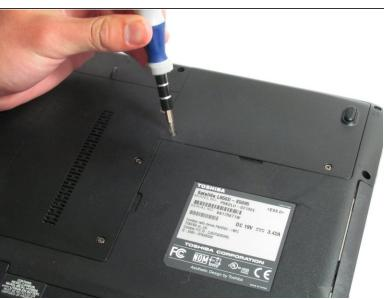
Unscrew the two screws holding the panel over the hard drive using a Phillips screwdriver. The panel is located on the top right of the laptop's underside.
