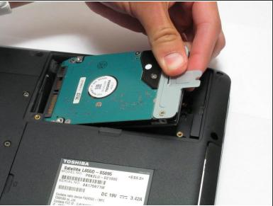
Remove the hard drive by pulling the tab upwards and sliding the hard drive out.
