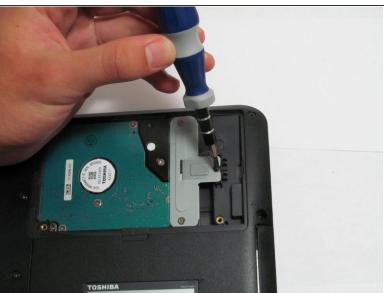
Remove the screw located under the plastic tab.
