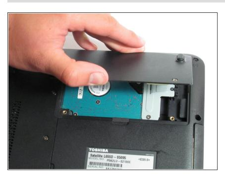
Remove the cover, firmly lifting from the indent. It is recommended that you leave the screws in the panel.
