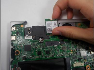
• Once the screw is removed, raise the WiFi card and slide it out from the motherboard.
