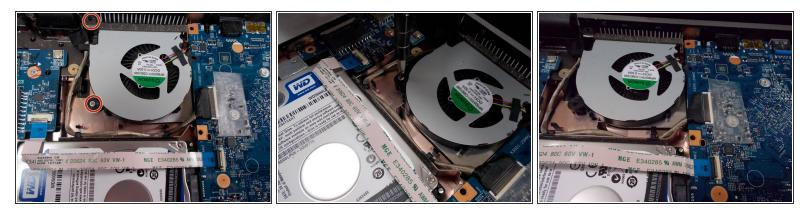
Using a Phillips #000 screwdriver, remove both 1.2mm screws that hold the fan in place.
