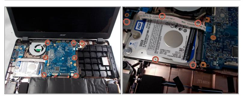
Remove twelve 1.2mm Phillips #000 screws from the motherboard, wireless LAN card, and hard drive.
