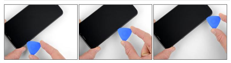
• Slide your tool along the left edge of the phone to separate the glue securing the display.
