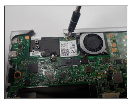
Use the Phillips #000 screwdriver to remove the screw holding the wifi card in place.
