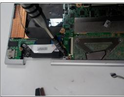
Use the Phillips #000 screwdriver to remove the three 3.5 mm screws which keep the motherboard in place.
