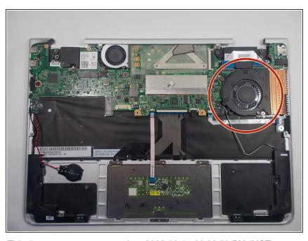
Locate the Cooling Fan in the device.
