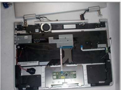
Carefully lift and remove the motherboard.
