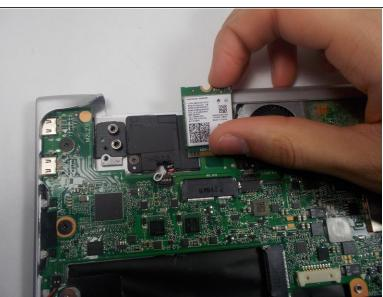
Once the screw is removed, raise the WiFi card and slide it out from the motherboard.
