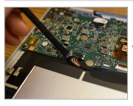
Using a spudger or other ESD-safe plastic tool, pry the thick plastic tape and foam top off the connector, just
