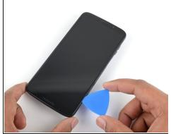
Slide the tool all along the right edge of the phone to slice through the adhesive securing the display.
