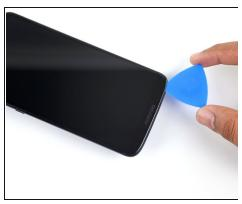
• Slice through the glue under the lower bezel.
