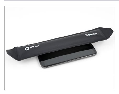
Heat the left edge of the phone to soften the adhesive securing the left edge of the display.
