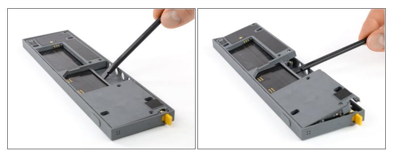
• Place a spudger in the cutout of the extension module to lift the midframe.
