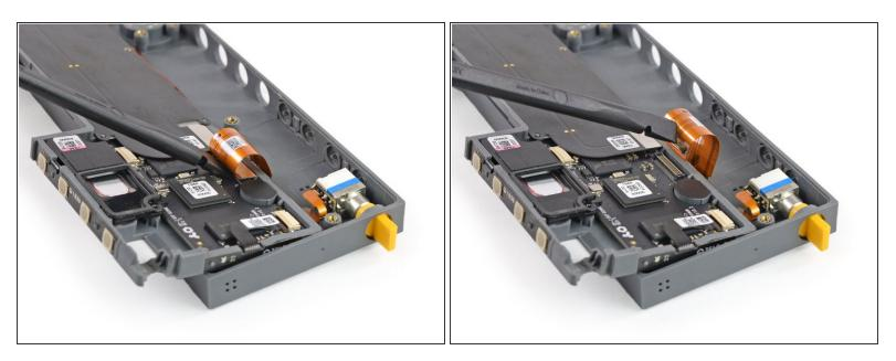
• Use the flat end of a spudger to disconnect the flex cable from the front panel assembly.
