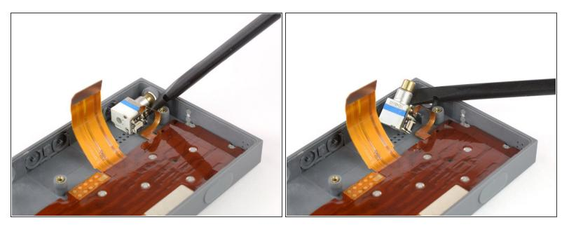
Use a spudger to lever up the axle of the volume potentiometer. This way it will clear the frame's cutout.
