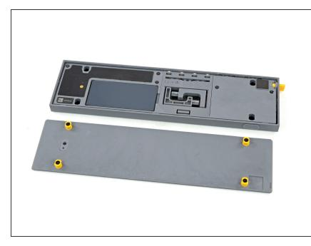
• Remove the bottom plate including the rubber feet.
