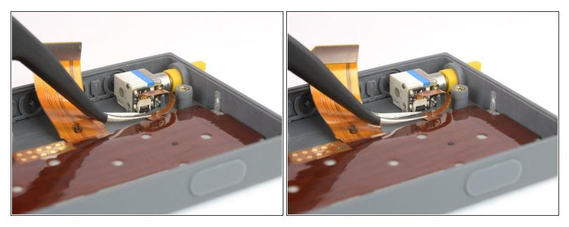
• Use one arm of a tweezer to lift the small black flap of the ZIF connector.
