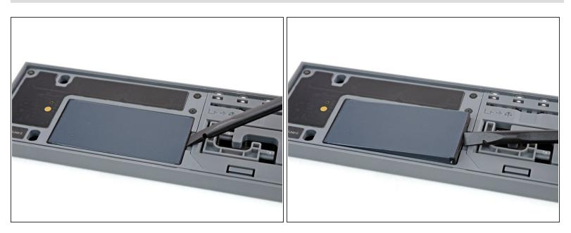
• Use your fingernail or a spudger to lift the battery on the right side where the notch is.
