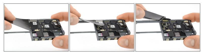
• Peel the highway flex cable off the midframe and remove it.
