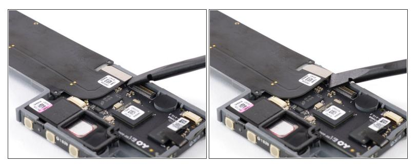
• Use a spudger to disconnect the highway flex cable from the DSP board.
