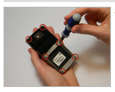
Remove the six 4.0 mm screws using the Phillips 00 screwdriver.
