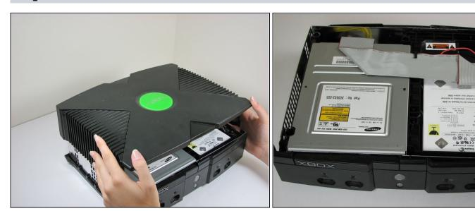
• Once the bottom and top shells are no longer attached, carefully turn the Xbox right-side-up, lift and remove the top cover.
