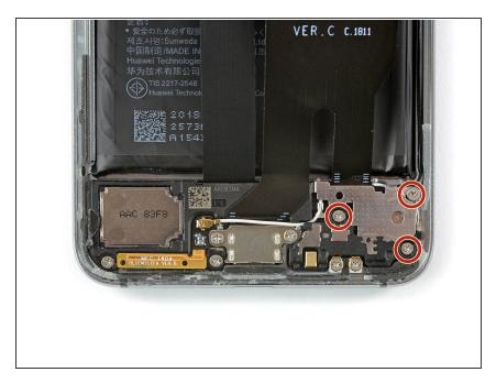
Remove the three Phillips #00 screws (3.2 mm length).
