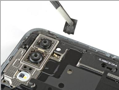
• Use a pair of tweezers to peel the black tape next to the rear camera off the motherboard cover.
