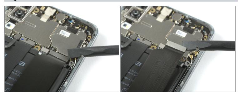
• Use a spudger to disconnect the main flex cable connector from the motherboard.
