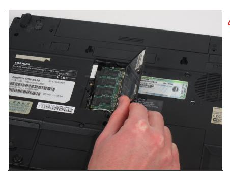
Carefully remove the cover to reveal the RAM compartment.
