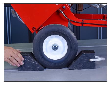
Place a wheel chock in front of a rear tire to keep the machine in place.
