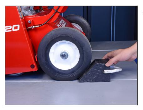
To prevent the over seeder from rolling during service, place wheel chocks behind a rear wheel.
