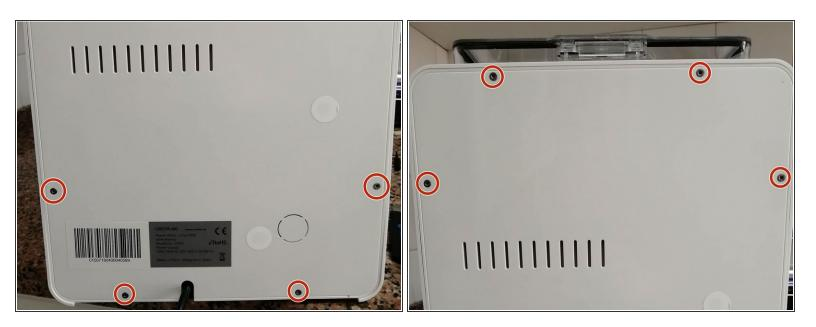
Using a T10 screwdriver, remove the eight screws located on the rear panel of the device (4 towards the bottom, and 4 towards the top).
