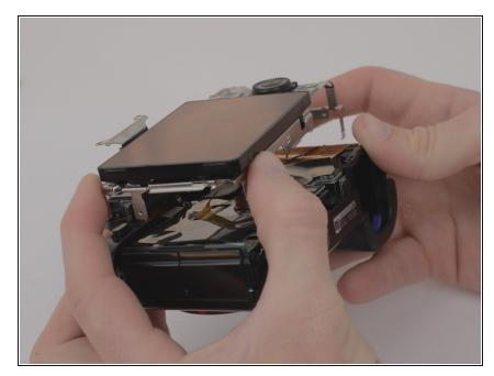
• Lift the metal plate and LCD screen away from the camera body.
