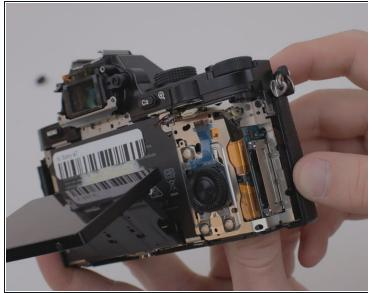
• Place the tweezers on the side of the circuit board and lift it from underneath so as to free it from the three retaining tabs.
