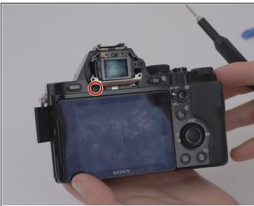
Remove the four M 1.5x2mm screws.
