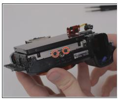
• Remove four M1.5x4mm screws using a PH00 Phillips screwdriver.
