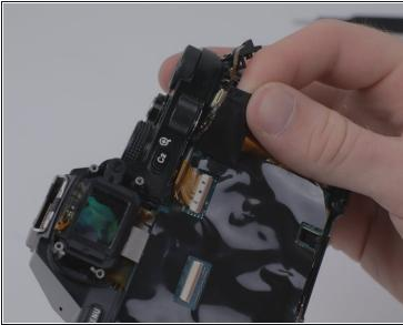
• Peel off the small adhesive tape located on the top right side of the motherboard.
