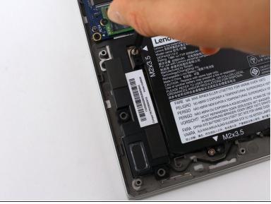
Remove the four 3.5mm Phillips #0 screws securing the battery.
