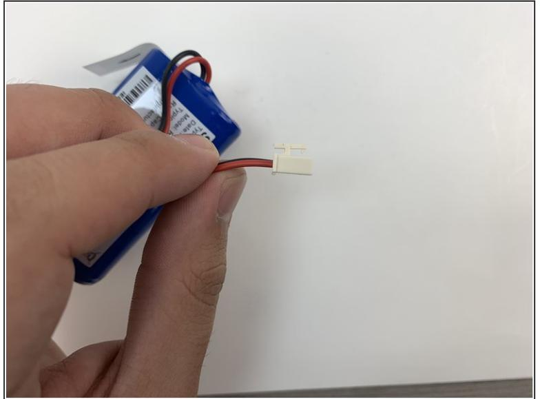
**⚠** Be careful when removing the connector, as the part can break if too much force is used.
