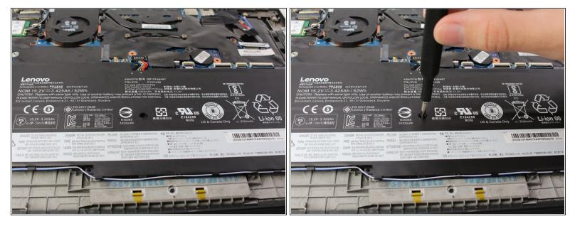
Remove the central 5 mm screw with a Phillips #1 screwdriver.
