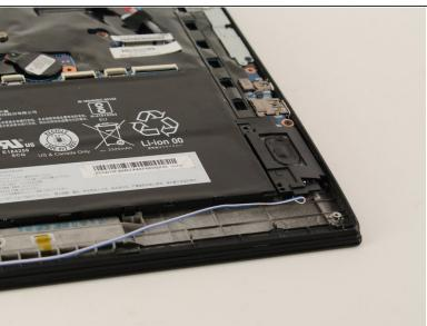
Unweave the blue and white wires from underneath the plastic tabs connected to the battery.
