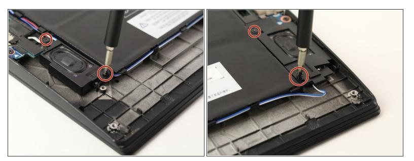
Remove the two 5 mm screws on each speaker with a Phillips #1 screwdriver.
