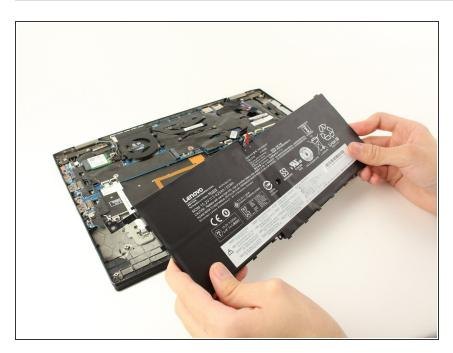
Lift the battery up and out of the computer.
