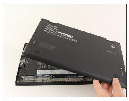
Lift the back cover up and off of the computer.
