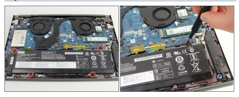
• Remove the four 4mm Phillips #1 screws securing the battery.
