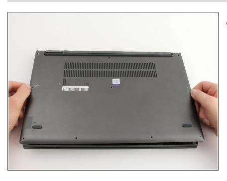
Pull the bottom cover up and away from the back hinges.
